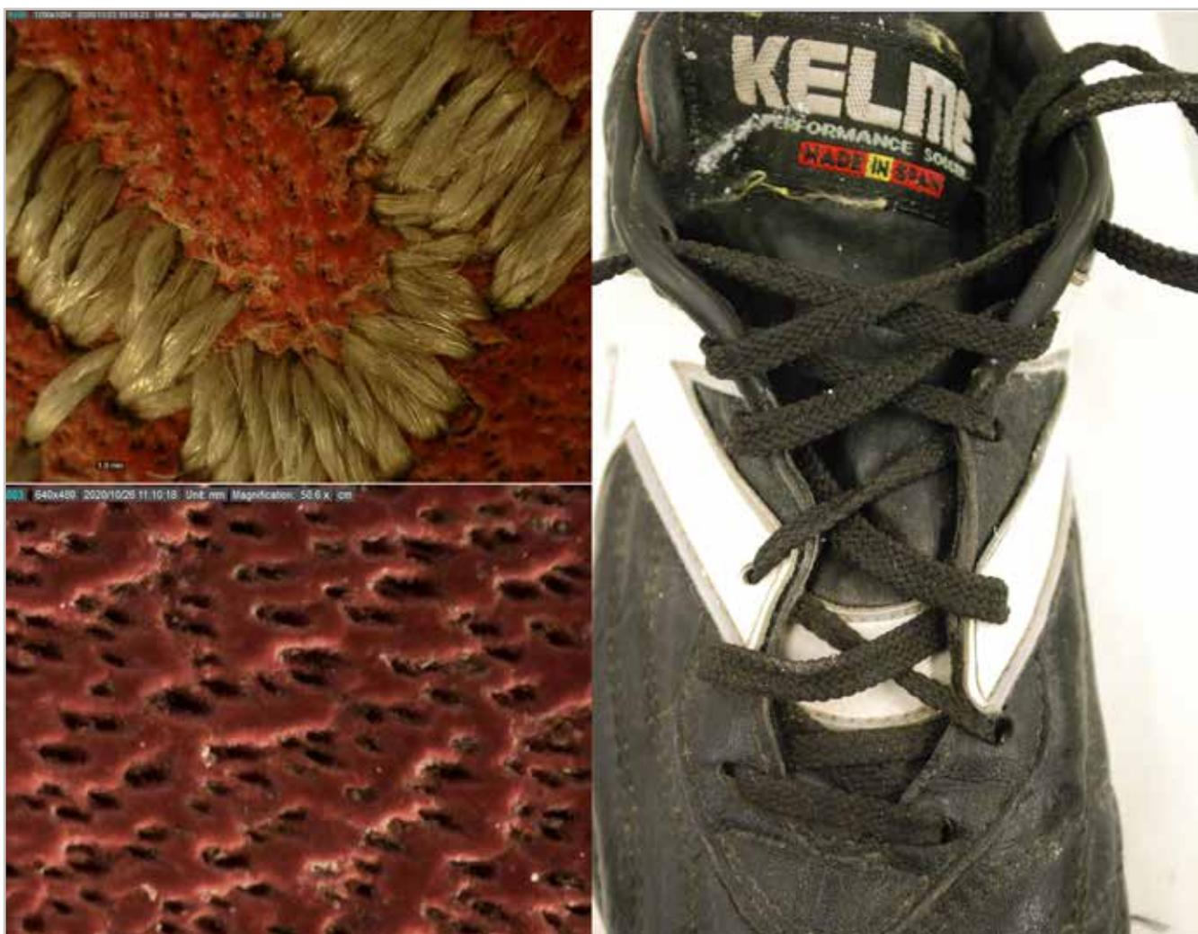
**Figure 4.-** Macro and microphotographs with visible light. Microscopic detail of the kangaroo leather, of the area of the footballer's name, at the turn of the tongue, and of the general condition of the laces. Before the intervention. Photograph: own authorship
